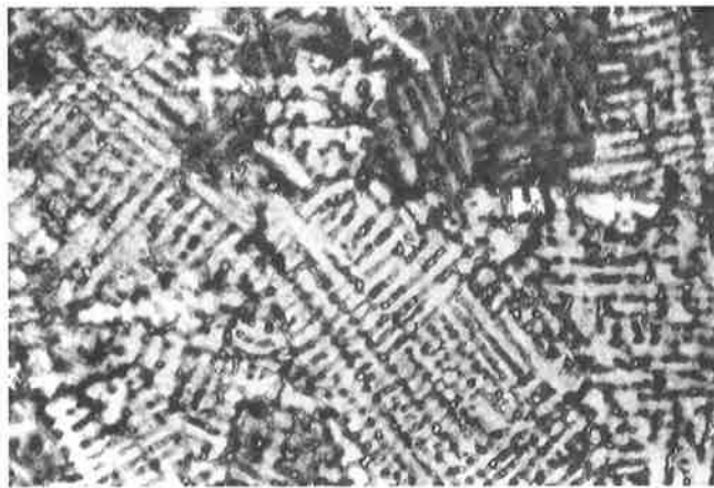
Fig. 65. Nr. 2210: partly worked foot of a Sanguisuga fibula; mainly cored dendritic structure with some incipient recrystallisation; the light, branched shapes are the cores of the dendrites; in a leaded low tin bronze. Scale 1:350.
